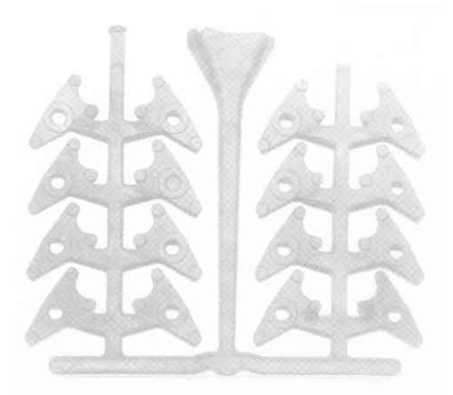
Fig. 3. Typical gating arrangement with bottom runner.
