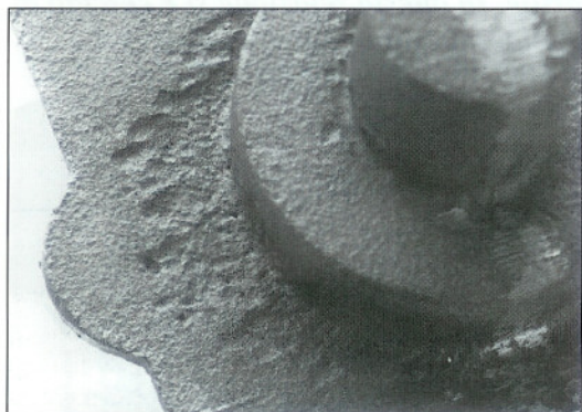
Fig.4 Surface defects associated to fluor contamination.
